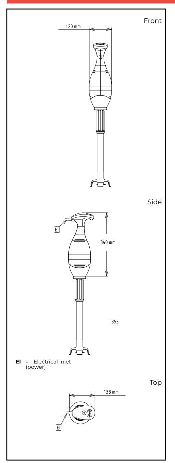
Electric Supply voltage: 220-240 V/1 ph/50/60 Hz **Electrical power max:** 0.75 kW 0.75 kW **Total Watts:** Capacity: Capacity (up to): 290 Litre Key Information: External dimensions, Width: 138 mm External dimensions, 120 mm Depth: External dimensions, Height: 965 mm **Shipping weight:** 5.96 kg
